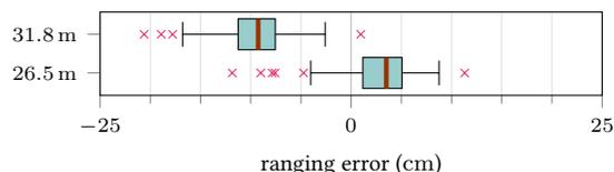
Figure 1: Error distribution of ranging with hydrophones at distances of approx. 26.5 m and 31.8 m (measured w. tapeline).
