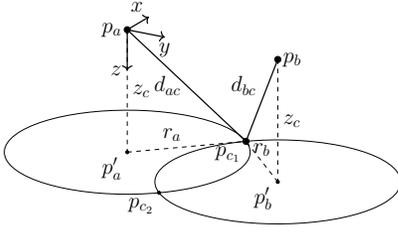
**Figure 2: Projection of  $p_a$  and  $p_b$  into the plane of  $p_c$ . To determine the solutions for  $p_c$  and  $\hat{p}_c$ , we use the measured distances  $d_{ab}$  and  $d_{ac}$ .**
