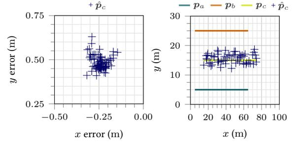
**Figure 3: Left: localization error during outdoor experiment with anchors at  $(25.4, 19.3)$ ,  $(-17.4, 20.8)$  and node at  $(0, 0)$ . Right: results of simulation with moving nodes ( $1 \text{ m s}^{-1}$ ) and localization every 2 s.  $\hat{p}_c$  denotes the estimated positions.**
